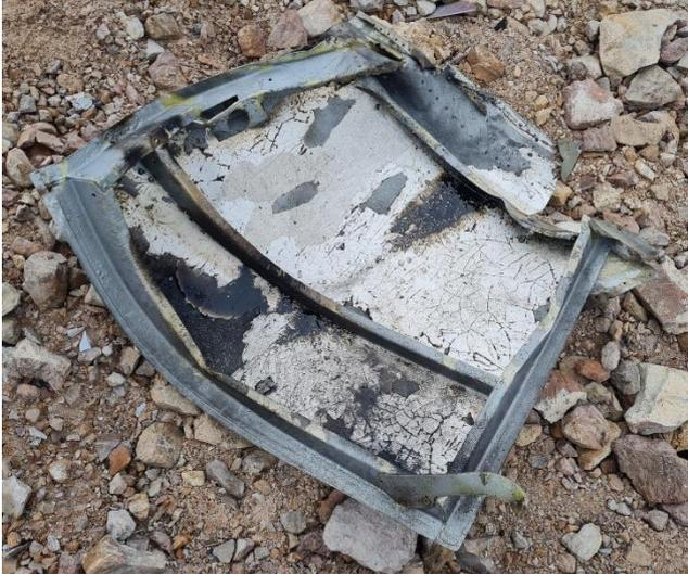
A photograph of a large, curved metal fragment of an aircraft fuselage, likely made of aluminum, lying on a rocky ground. The fragment is heavily damaged and shows signs of impact.                    | Фрагмент обшивки фюзеляжа                           |
