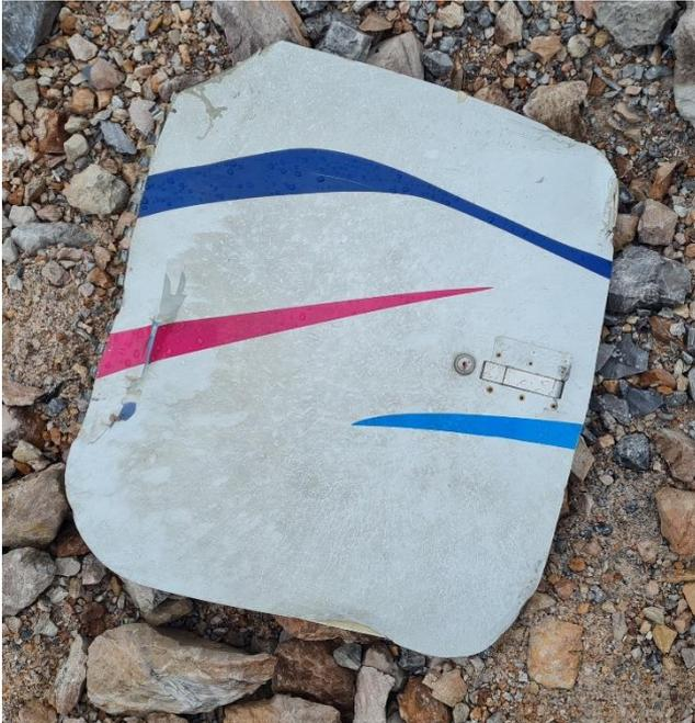
A photograph of a large, rectangular, light-colored metal lid, likely from a baggage compartment, lying on a rocky ground. The lid has blue and red stripes and a small metal latch or fastener.       | Крышка багажного отсека                             |
