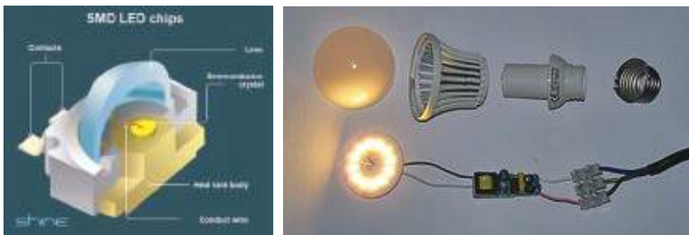
Figure 49. Construction of various LED lightbulbs.
