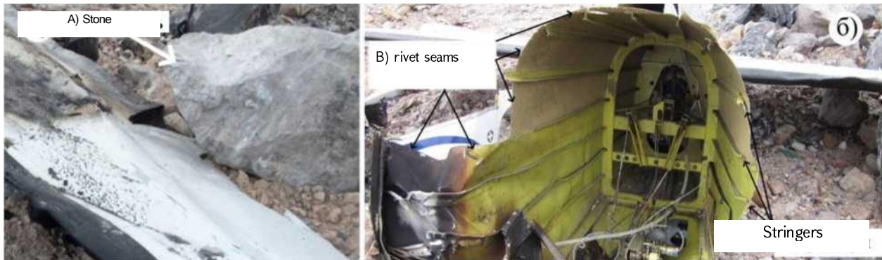
Picture 6. Image: of a stone - a), destruction and deformation of framework elements of rear end of AC – b)
